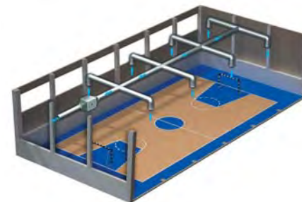
VS fan gym ventilation example
